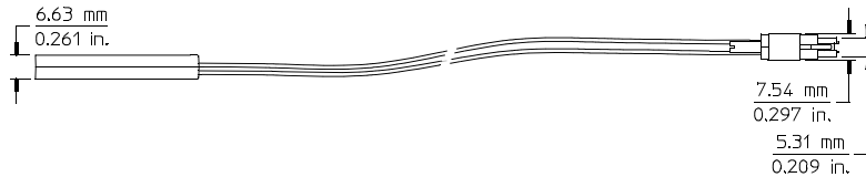
Figure 10 E5398A probe dimensions
